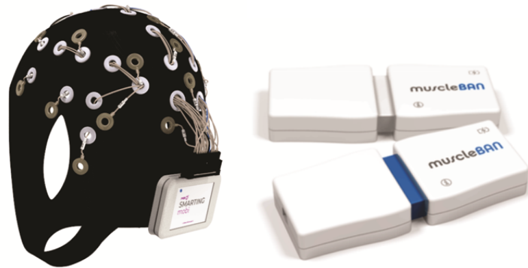
Fig.3.1.1.1: EEG cap and EMG sensors
