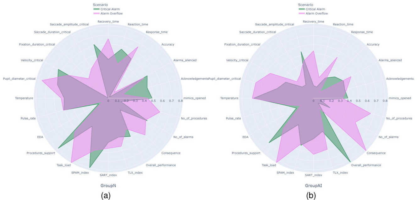
Figure 27. Radar plot between scenarios critical alarm (green) and alarm overflow (violet) for (a) GroupN and (b) GroupAI.
